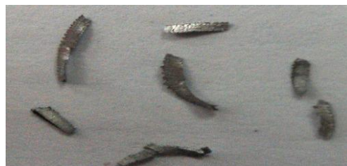
Figure 1 Elemental chips on cutting conditions V=250 m/min, F= 0.15 mm/rev, D.O.C 0.3 mm
